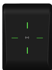
Green LED Access granted
