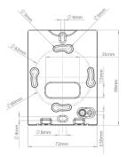
**Back plate** Back plate compatible with UK, EMEA and US standard and most electrical gang mountinas
