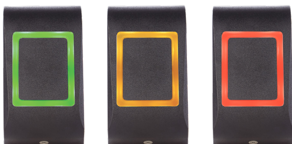
Green LED Access granted
